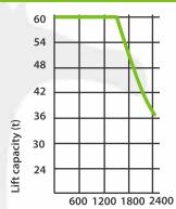
Distance to centre of load (mm) From the surface of the fork The lift capacity is with vertical mast
